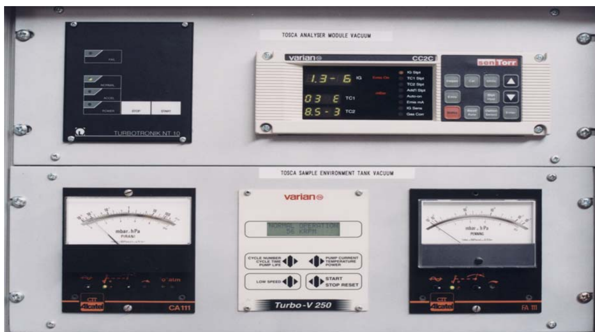
Figure 5.1. The vacuum gauges on TOSCA
