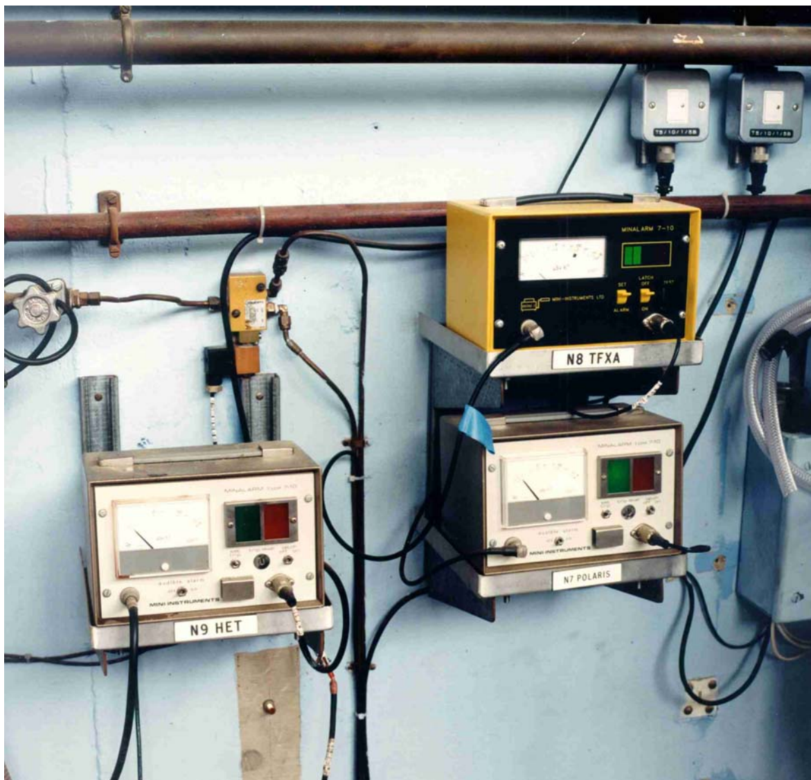
Figure 2.9: The radiation monitor on the target station wall. Tosca's is labelled "N8 TFXA" (upper right). 01RC1868
