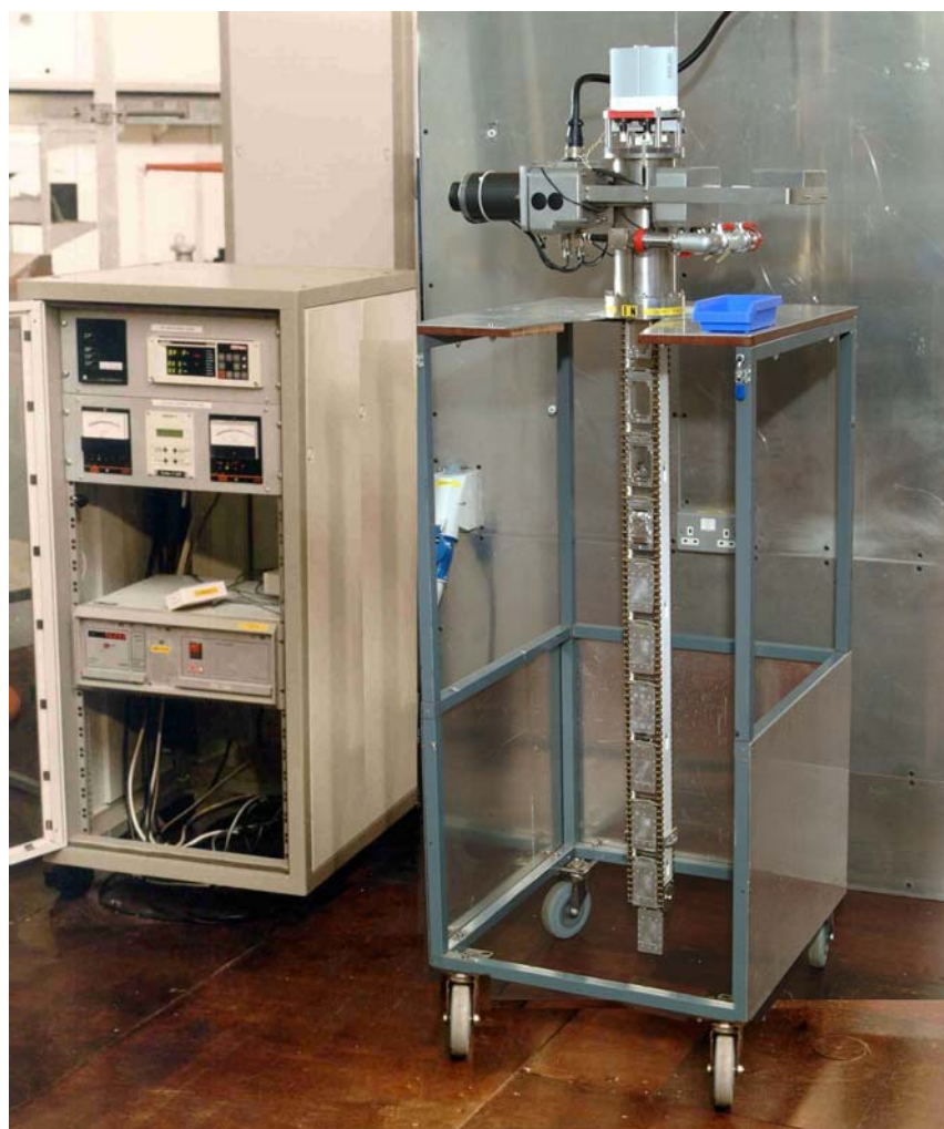
Figure 2.3: The 24 position samplechanger in its cradle (right) and its controller (bottom panel in electronics rack on the left).
