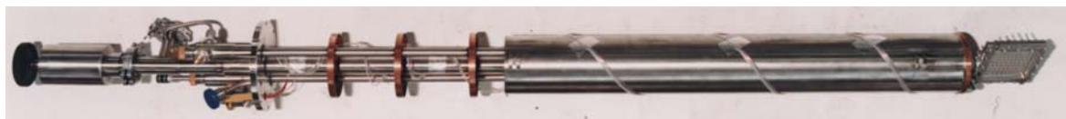
Figure 1.3: The liquid helium centrestick for use on TOSCA.
